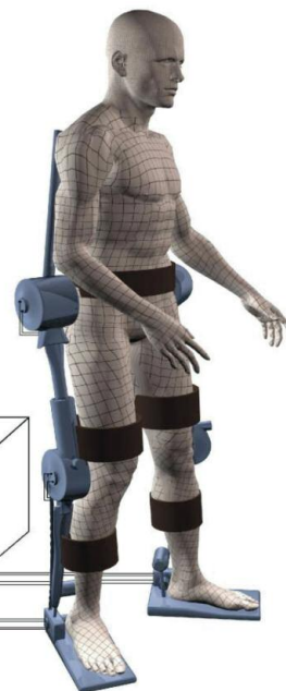
The patented Intelligent Exoskeleton for Spinal and Lower Extremities Rehabilitation
